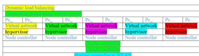
Fig. 7 Schema for Driving a distributed computing systems based on cloud computing technology
